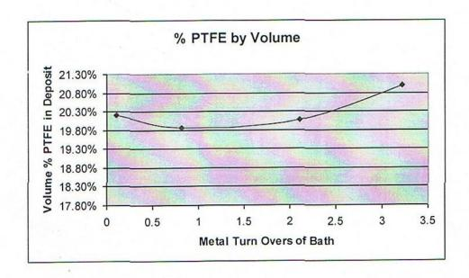
The trial work was done with a commonly used concentration of six grams per liter of PTFE dispersion in the plating bath. As is known in the industry, the percentage of PTFE in the deposit can be readily increased by increasing the concentration of PTFE dispersion in the bath. This was confirmed in the new system in additional trials where greater than twenty-five percent by volume PTFE was achieved by a relatively small increase in PTFE concentration in the plating bath.
