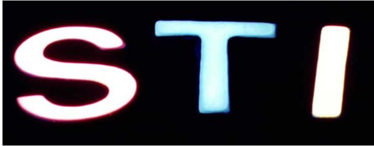
Photograph 1 – Three metal letter substrates coated with three different varieties of composite EN with light emitting particles and photographed under ultraviolet light to reveal red, blue, and white luminescence.
