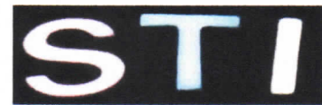
Aluminium letters coated with three different versions of Illumi-Layer and photographed under ultraviolet light.
